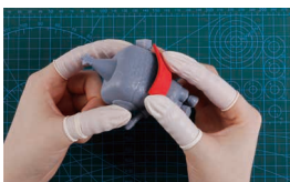
砂纸和海绵砂纸进行精细打磨 然后用清水和抹布洗去表面粉尘 Sand with sandpaper and sponge sandpaper, then wipe off the dust with water and a cloth
