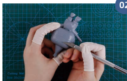
美工刀切削细微支撑 Cut off the tiny supports with a craft knife
