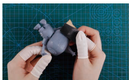
用斜口钳修剪支撑 Remove the supports with snip
